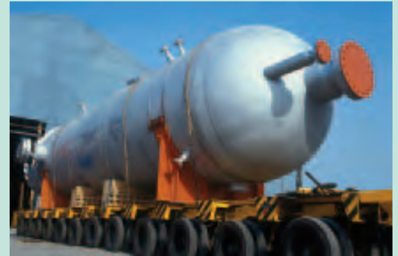
ISGEC supplied this High Pressure Separator Vessel to SNC Lavalin, Canada. This Vessel, having Stainless Steel weld overlay is being used in a Gas Processing Plant that they built for Petroleum Development Oman. The vessel weighs 210 Tonnes.
